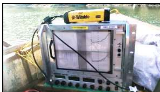
Echo-sounder & GPS used during the survey
