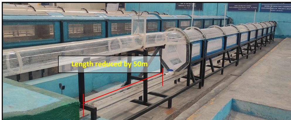
Model of desilting chamber of Kholongchhu H. E. project, Bhutan after reduction in length
