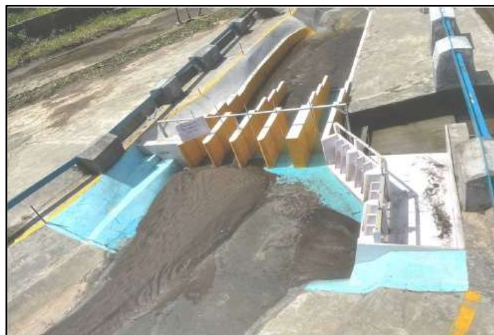
View of Teesta VI physical model after flushing operation
