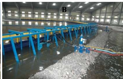
A) Multipurpose Wave Basin Hanger B) Wave Generation System C) RSWG control and DAS Cabin with SCADA System
