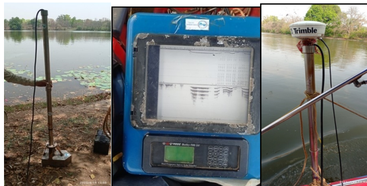
Echosounder sensor with readout unit and DGPS antenna
