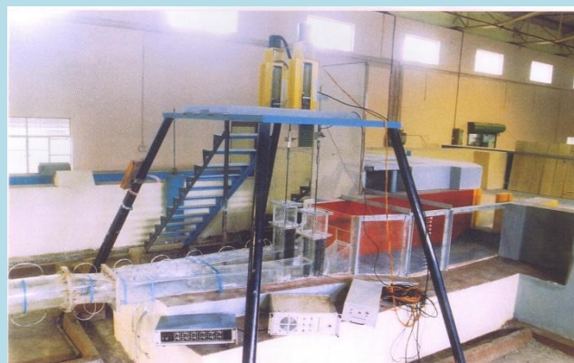
Service gate installation at IBPT model, Sardar Sarovar, Gujarat
