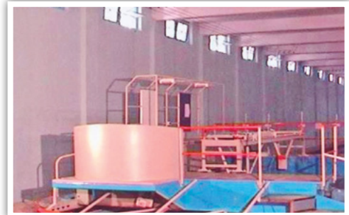
Front view of Current Meter Rating Trolley
