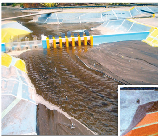
Reservoir flushing model
