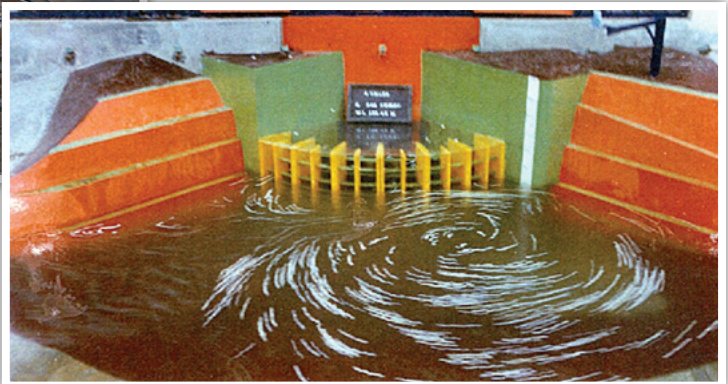
Vortex formation in pumping mode at Srisailem Project
