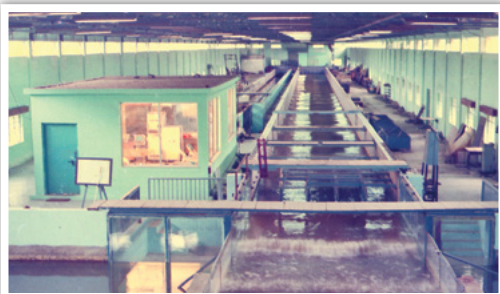
Random sea wave generating flume
