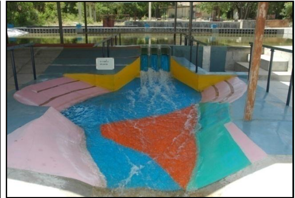
Modified Design of Spillway Tail Channel
