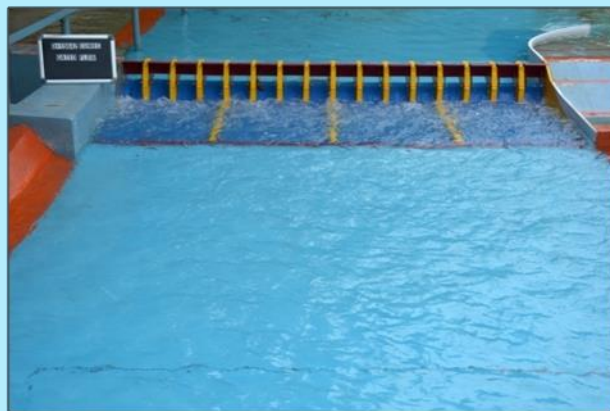
Physical model studies for spillway & energy dissipator
