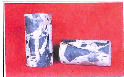
Fig. 15 – Cores after grouting
