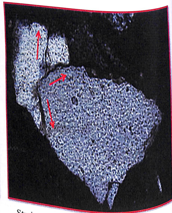
Strained quartz --- three-way undulatory cracks under microscope
