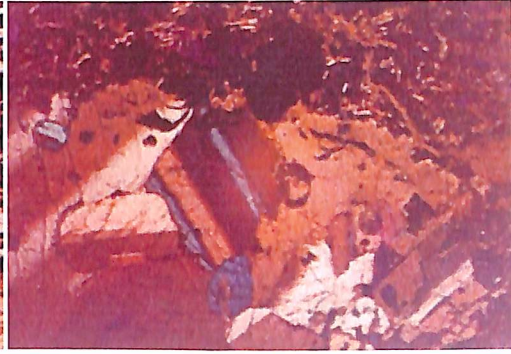
Porphyritic basalt – corroded boundaries of plagioclase and altered minerals with volcanic glass
