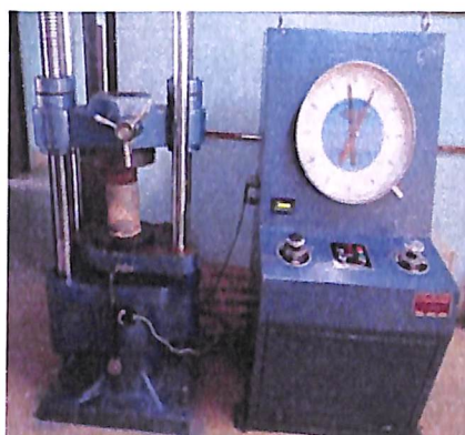
Fig. 2.42 Compression test set up
