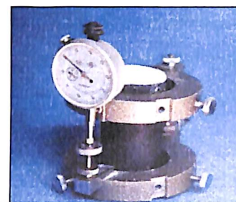
Fig. 3– Set up for modulus of elasticity
