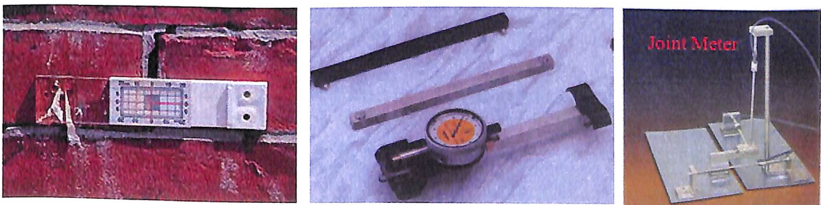
Fig. 2.3 Typical Crack meter and joint meter
