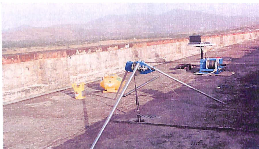
Fig. 2.31 Schematic Setup of Borehole Logging
