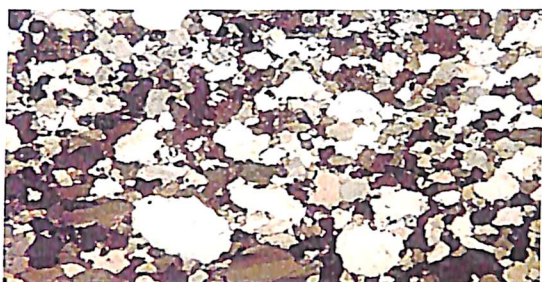
A: General bedding and interlocked boundaries of grains showing Mosaic Texture
