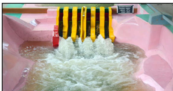
Flow Conditions downstream of spillway (Q = 6,900 m 3 /s, gated operation of spillway)
