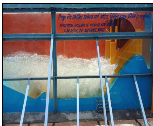
Flow condition downstream of spillway for Ungated Operation of Spillway for the Discharge of 9122 m 3 /s (100%) at RWL El. 191.45 m
