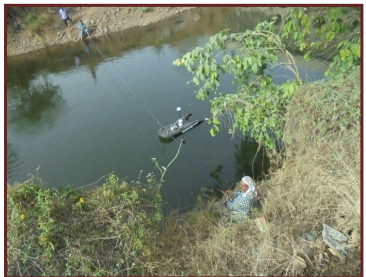
Discharge measurement by ADCP at the D/s of Godbole Gate
