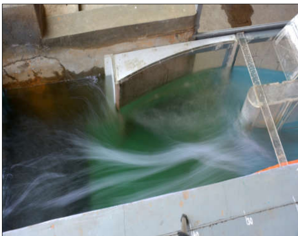
Flow conditions in the approach channel
