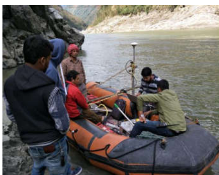
Survey Boat with Beacon DGPS and Echo Sounder for Hydrographic Survey
