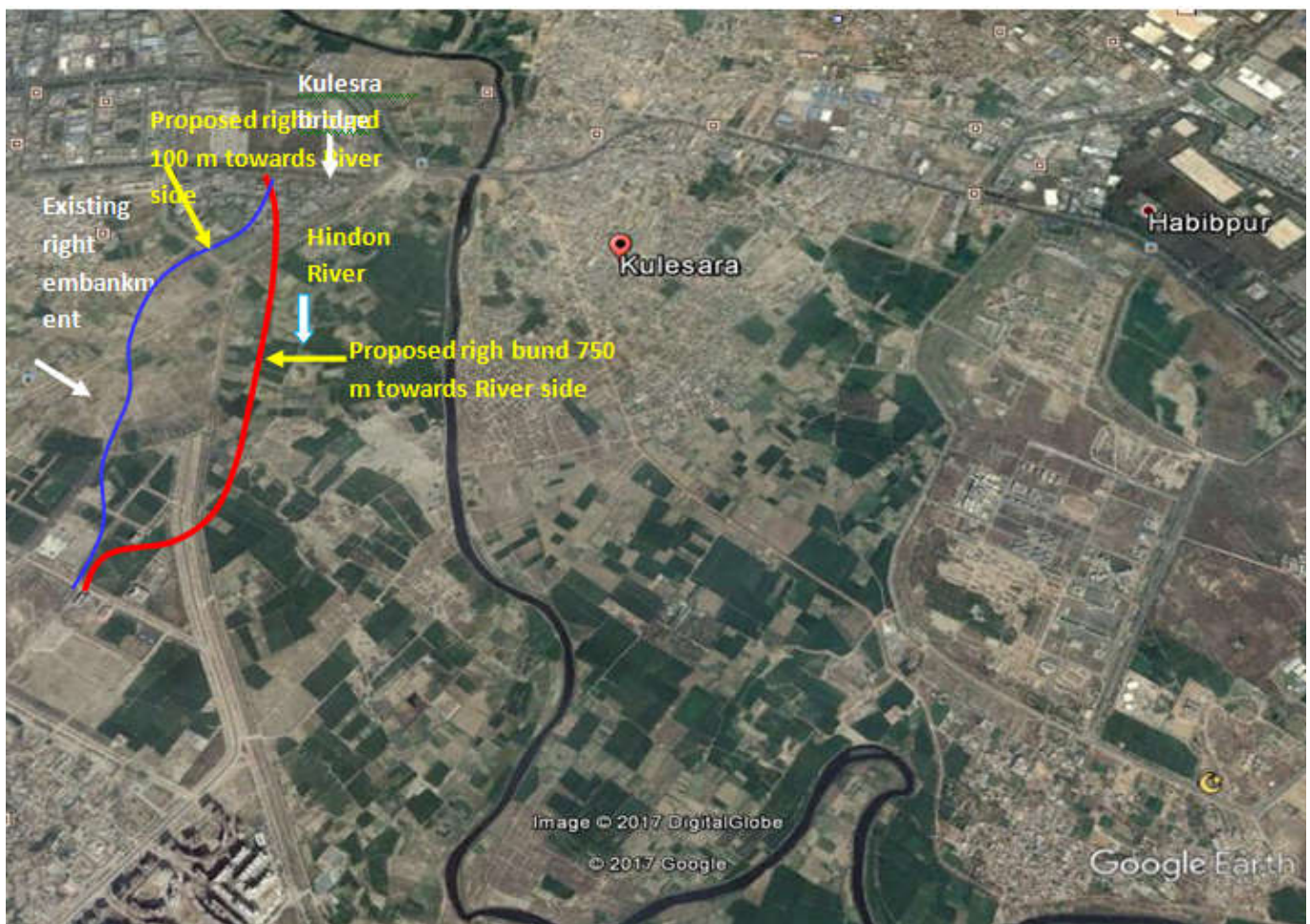
Plan showing study area with existing bund and proposed bunds along River Hindon 750 m
