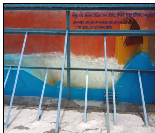
Performance of Stilling Basin for Gated Operation of Spillway for the Discharge of 4561 m 3 /s (50%) at FRL El. 192.024 m
