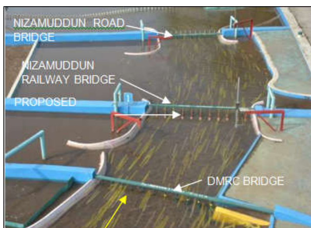
Flow pattern in the vicinity of proposed Railway bridge for Well foundation for Q=7022 m 3 /s
