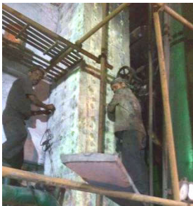
In-situ Ultrasonic and Rebound Hammer tests in progress
