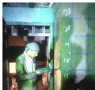
In-situ Ultrasonic and Rebound Hammer tests in progress
