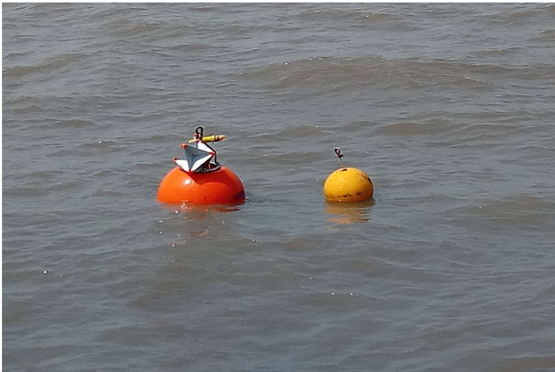
Acoustic Doppler Current Profiler (ADCP) Deployed near jetty of M/s Petronet LNG Ltd. at Dahej, Gujarat
