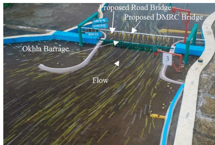
Flow pattern in the vicinity of proposed Road bridge 35 m downstream of DMRC bridge across river Yamuna at Delhi
