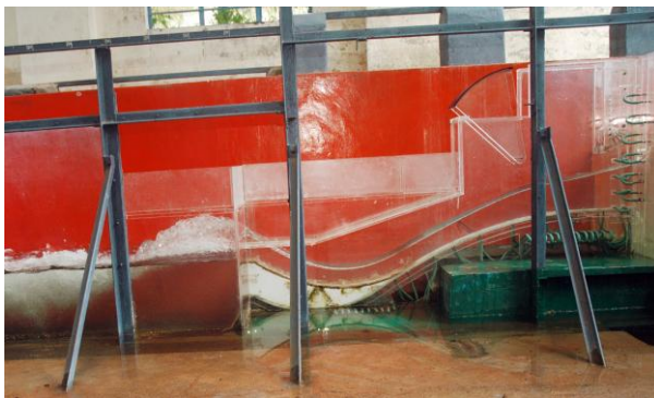
Flow conditions for ungated operation of spillway, Q=5750 m 3 /s (50%) at RWL El. 1181.47 m
