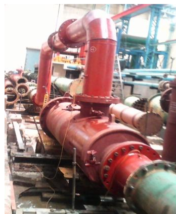
Head loss testing of heavy duty filter for NTPC
