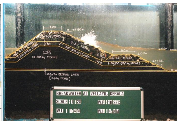
Wave flume test for breakwater
