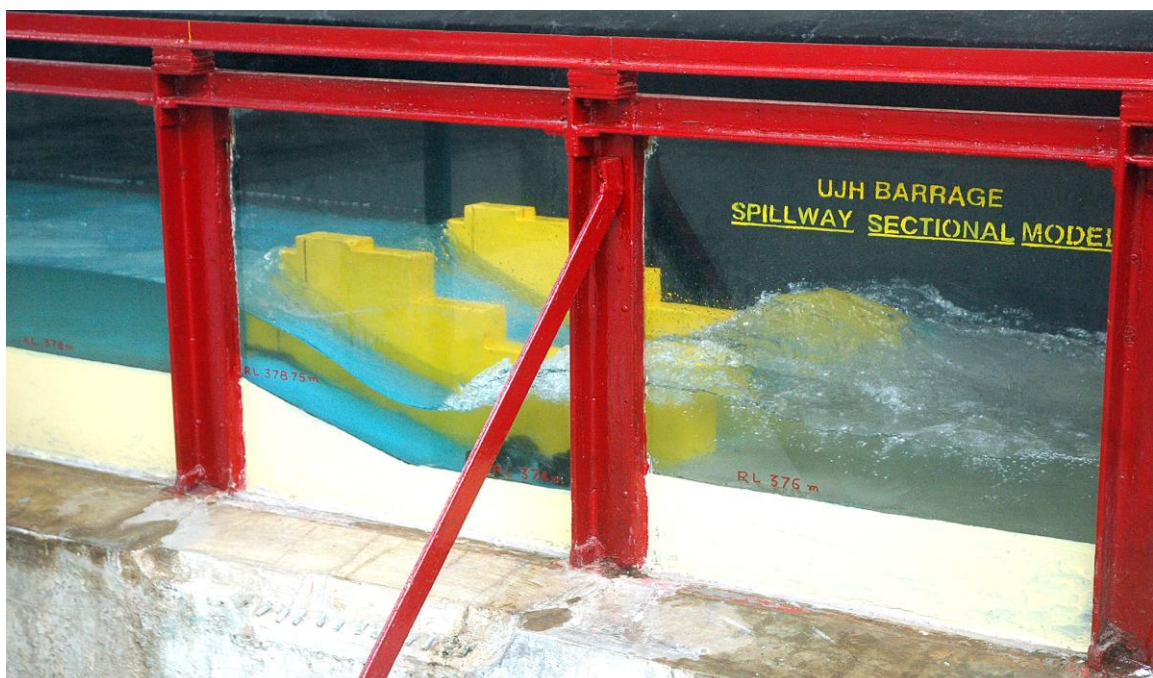
Flow conditions/ water surface profile for a discharge intensity of 37 m 3 /s
