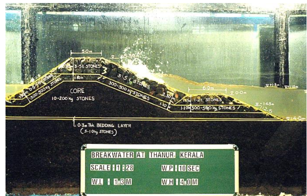
Wave flume test for breakwater
