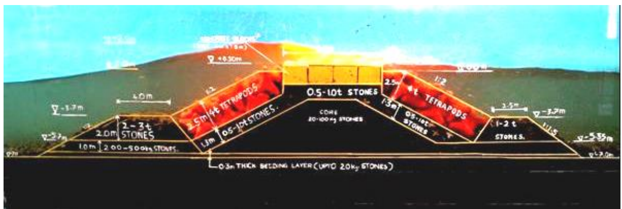
Wave flume studies for the design of offshore reef at Ullal
