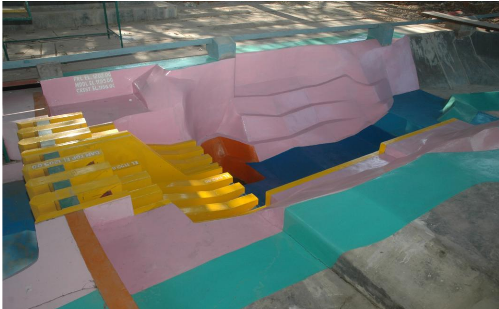
Dry model showing dressed downstream portion
