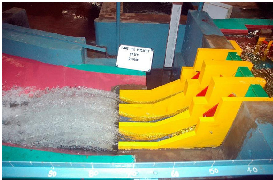
Flow conditions downstream of the spillway for partial gate operation Q=5000\text{ m}^3/\text{s} , FRL El. 245.15 m
