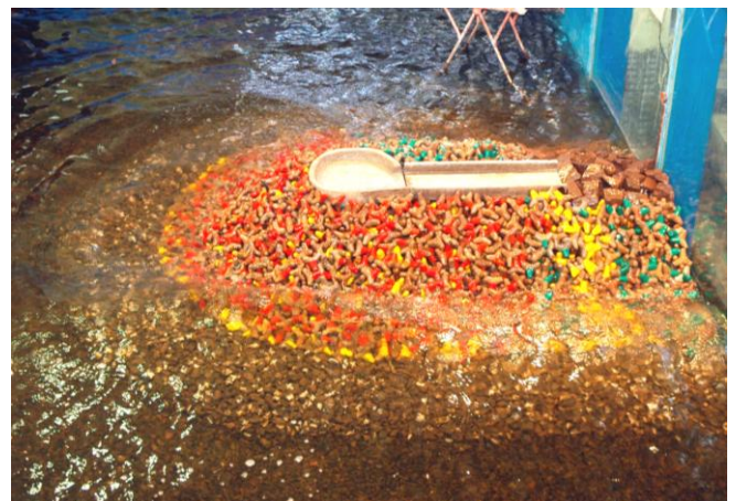
Wave flume testing of roundhead of breakwater
