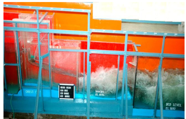
Flow conditions over the spillway and energy dissipator
