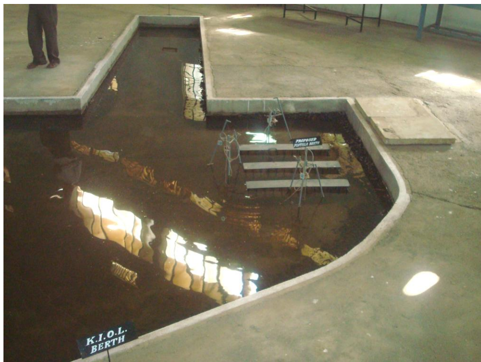
Photo showing Flotilla Jetties simulated on the model
