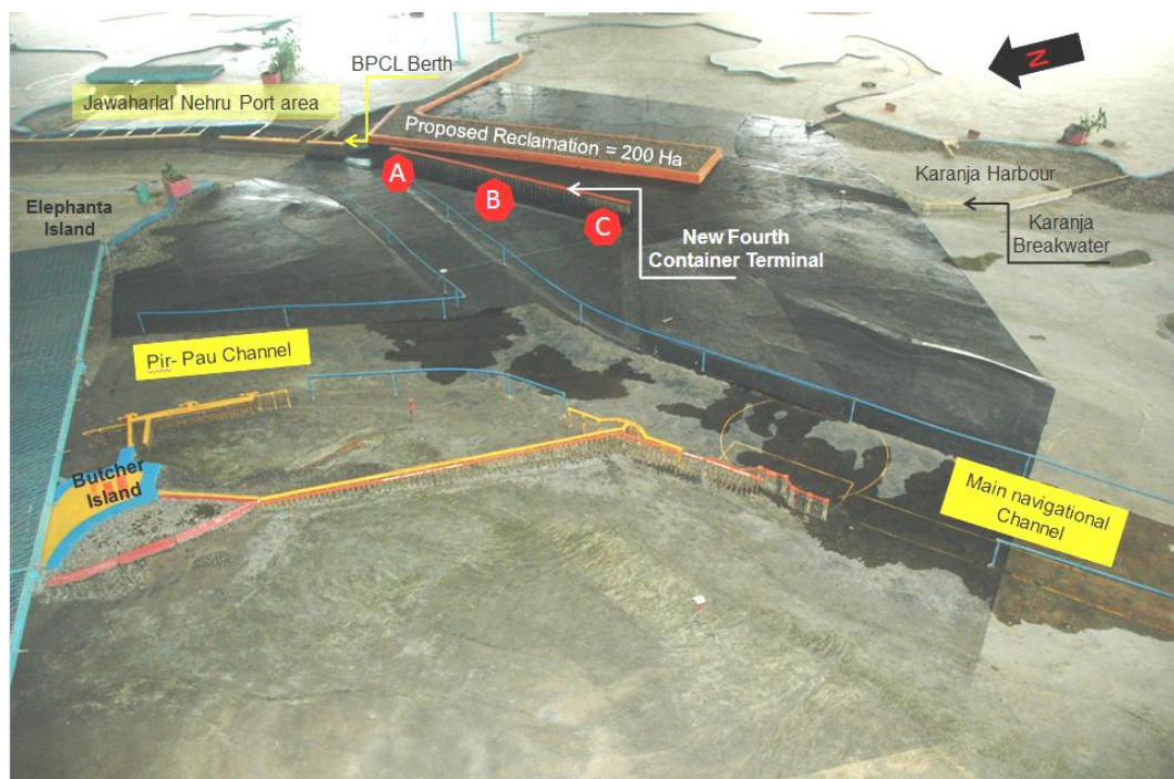
Layout of 4 th container terminal studied on physical model (2000 m long terminal in one line)
