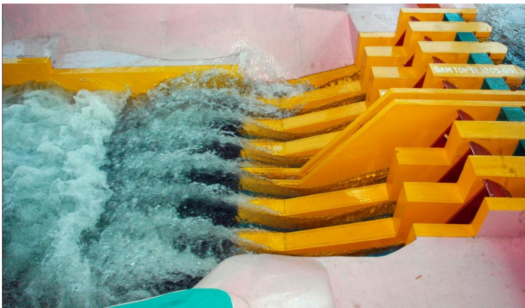
Flow condition downstream of spillway for 15,800 m 3 /s
