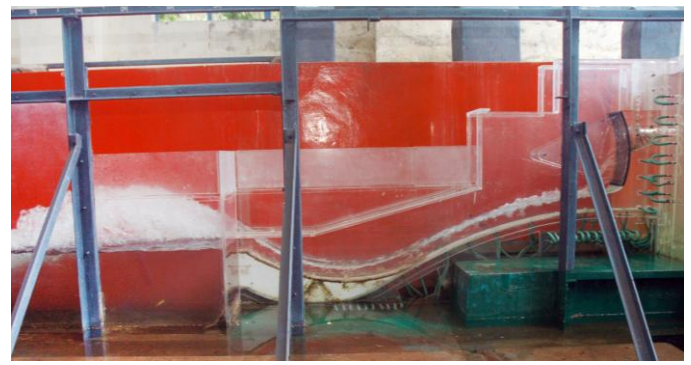
Flow conditions for gated operation of spillway, Q=5750 m 3 /s (50%) at FRL El. 1202 m
