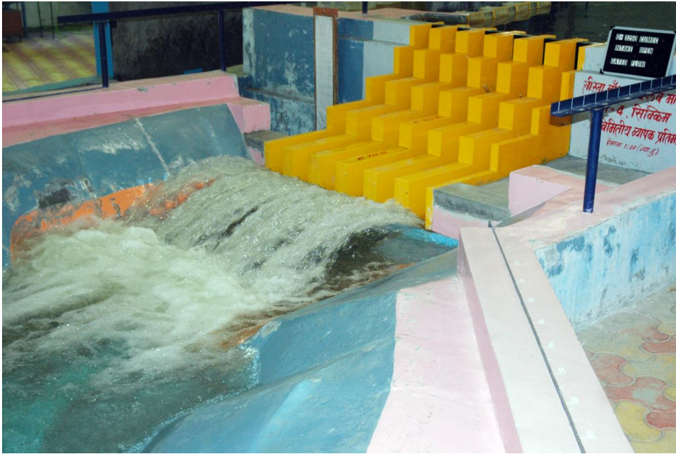
Performance of ski-jump Bucket for gated operation of spillway Q=3250 \text{ m}^3/\text{s} (25%) at FRL El. 755 m
