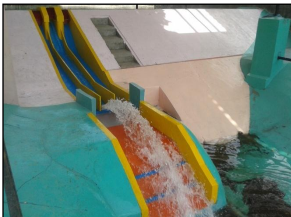
Flow conditions downstream of spillway, Q= 675 m 3 /s (One gate in operation RWL El. 1643.5 m)
