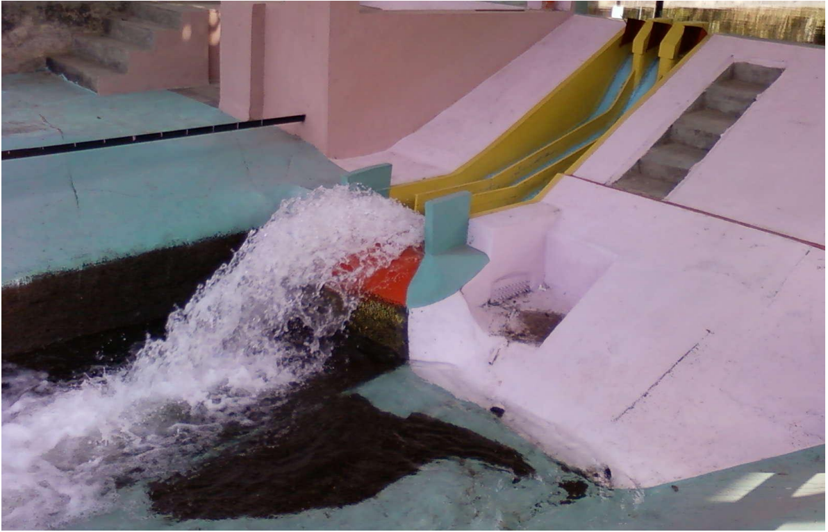
Flow conditions downstream of spillway, Q= 1643 \text{ m}^3/\text{s} (FRL El. 1643.5 m, Gated)
