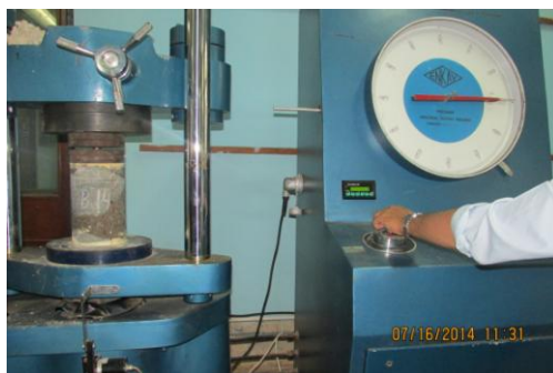
Compression test under progress
