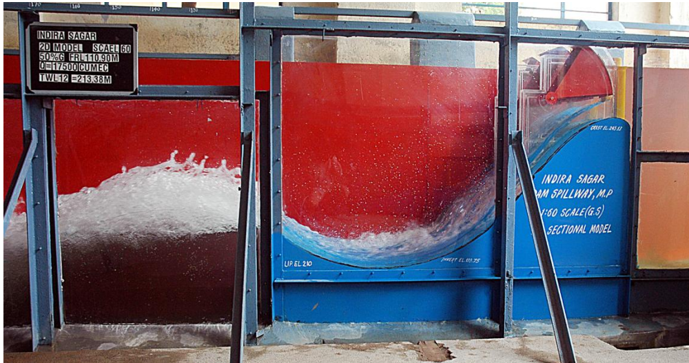
Flow condition for gated operation of main spillway Q=17769 \text{ m}^3/\text{s} (50%) at FRL El. 262.13 m
