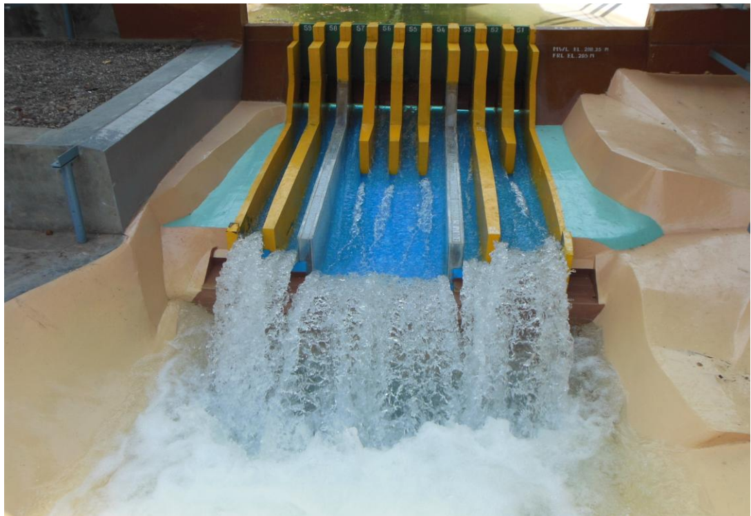
Performance of EDA for Q = 17,500 \text{ m}^3/\text{s} operating at FRL El. 205 m
