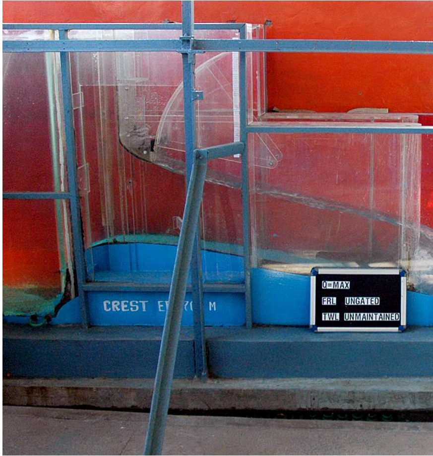
Flow conditions in the vicinity of the breast wall ( Q = 12000 \text{ m}^3/\text{s} at FRL El. 1747 m with ungated operation of spillway)
