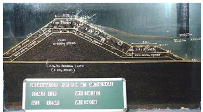
Wave flume test for breakwater
