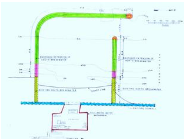
Layout of breakwaters
