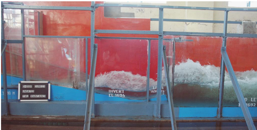
Flow conditions over the spillway and energy dissipator ( Q = 8500 \text{ m}^3/\text{s} , Ungated operation of spillway)
