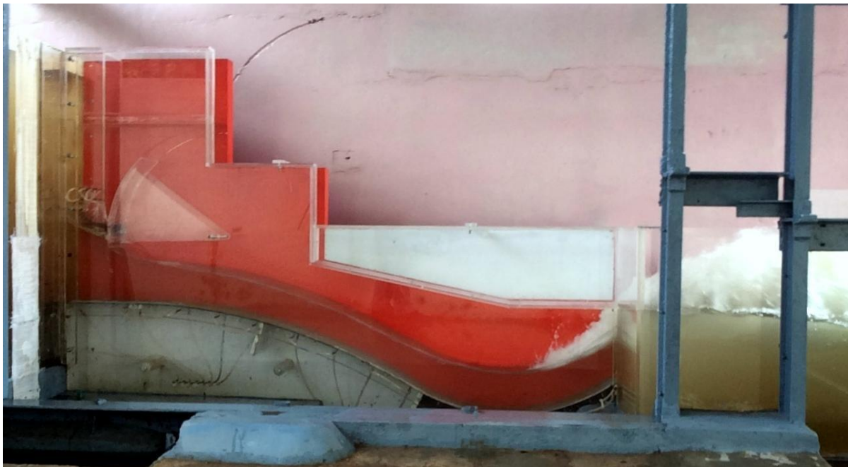
Performance of ski-jump bucket ( Q= 16,023 \text{ m}^3/\text{s} (100%), gated
