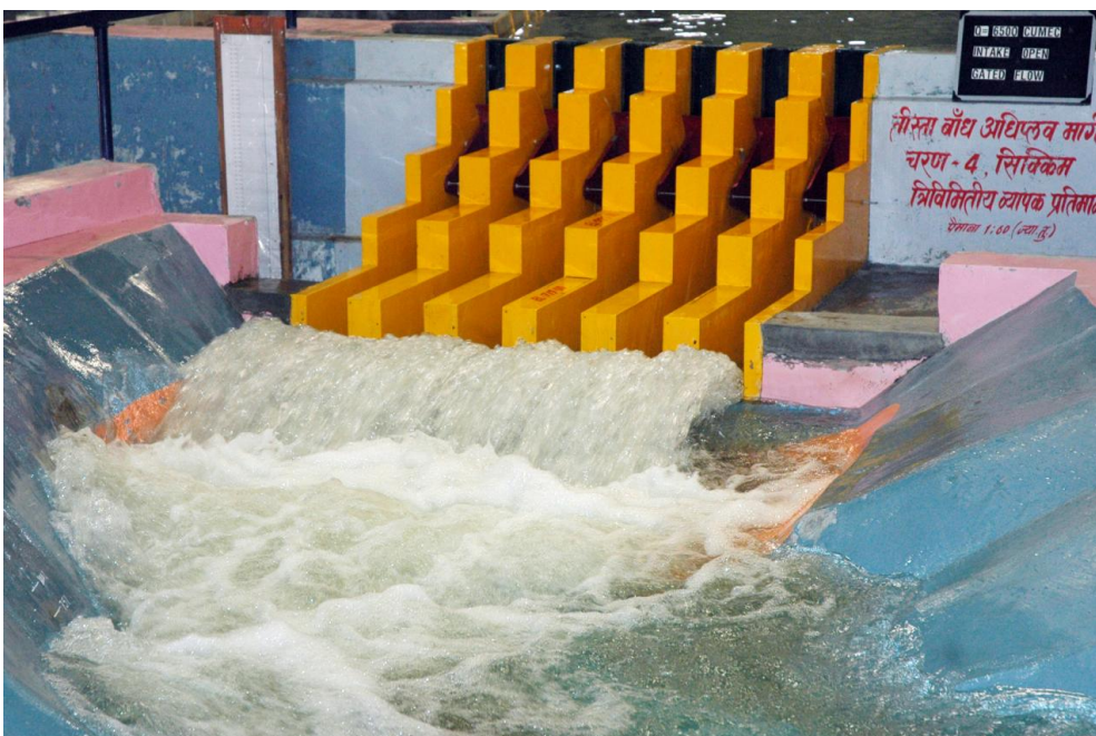
Performance of ski-jump bucket for gated operation of spillway Q=6500 \text{ m}^3/\text{s} (50%) at FRL El. 755 m
