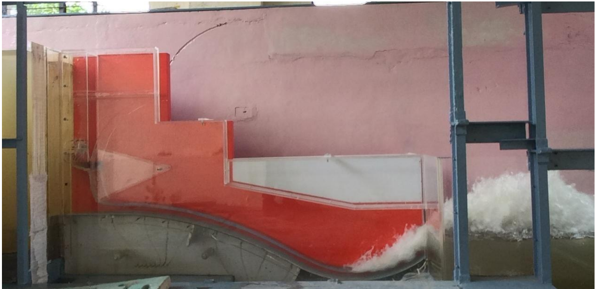
Performance of ski-jump Bucket ( Q= 4,006 \text{ m}^3/\text{s} (25%), gated
