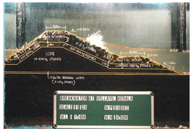
Wave flume test for breakwater
