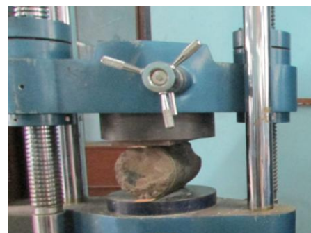
Split tension test assembly
