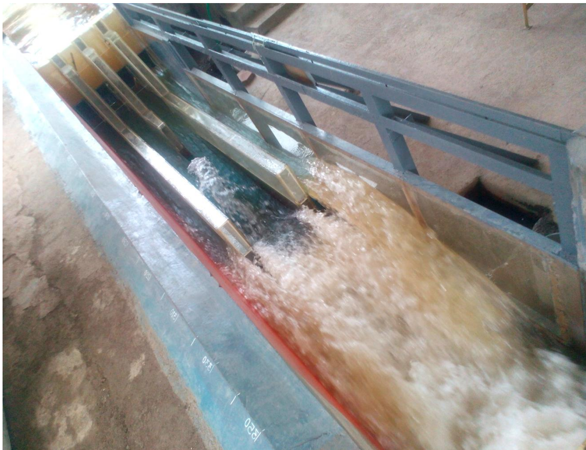
Performance of Ski jump bucket for Q = 35,000 \text{ m}^3/\text{s} at FRL El. 205 m
