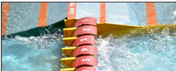
Flow Condition for the Original Design of the Upstream Divide Wall and Downstream Training Wall
