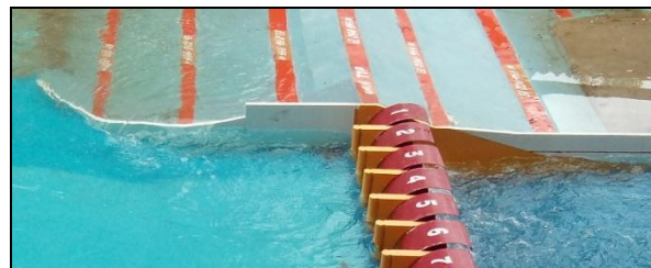
Flow Condition After the Provision of Upstream Curved Guide Wall
