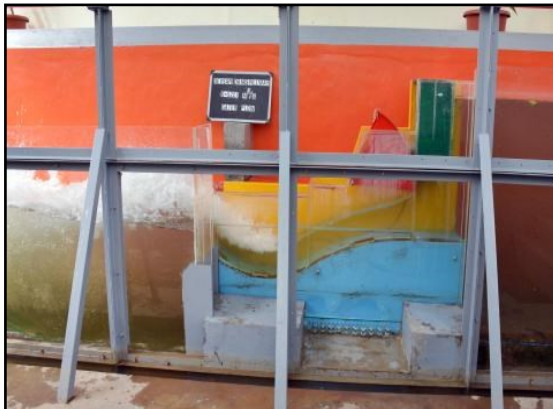
Flow condition in ski-jump bucket
