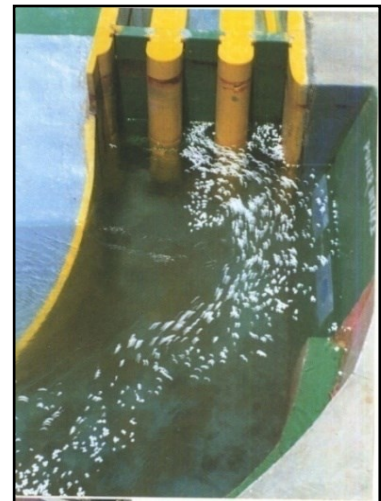
Non-Uniform approach flow conditions
