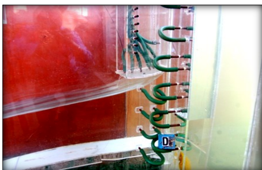
Flow condition near original roof profile
