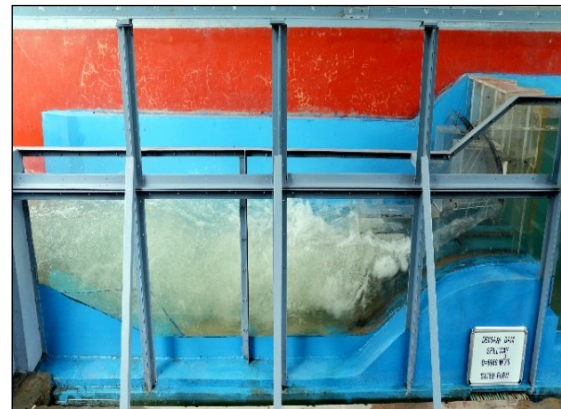
Flow condition in Stilling basin
