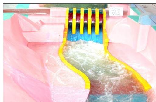
Flow conditions in the stilling basin
