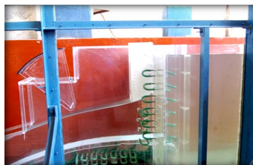
Flow condition near modified roof profile
