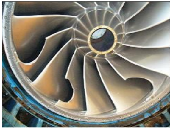
a) Runner with cracked vanes in 2004
