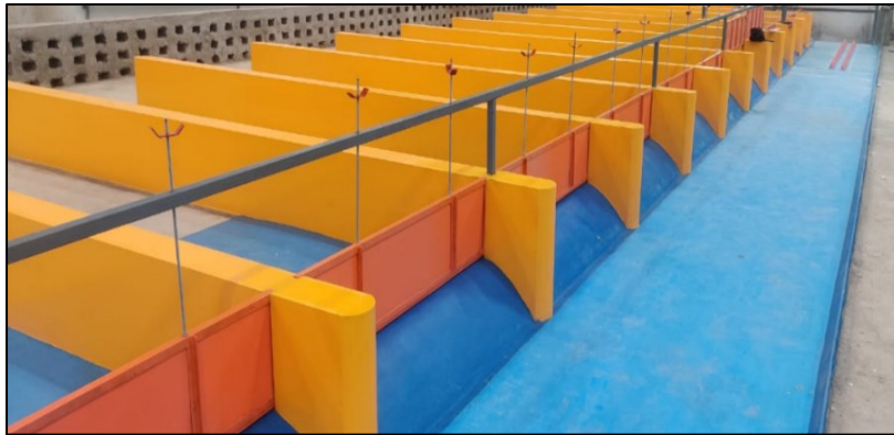
Physical model of Kalpasar Dam spillway, Gujarat
