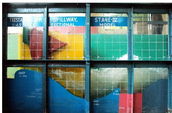
Flow conditions in the bucket
