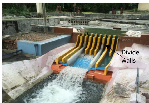
Model view showing spillway operation for Subansiri Project with provision of divide walls
